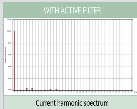
Figure 9: Current Harmonics Spectrum
